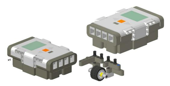
Attach the parts from Step# 3 to the NXT at the protruding connector pegs.
