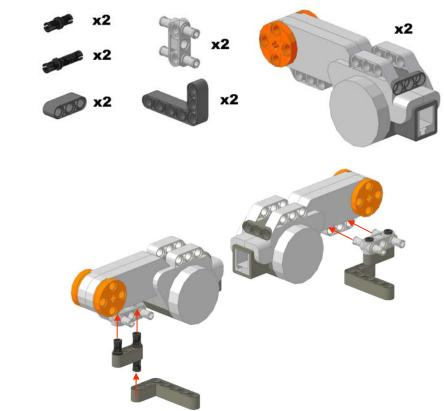
Attach a four pin axle joiner to each of the NXT motors. In 1 hole of the 4 pin connector attach a pin and in the other hole attach an extended pin. Attach the short beam to both pins and the bent beam to the extended pin.
