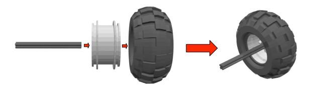
Assemble  $\underline{2}$  rear wheel assemblies using a 6 stud axle, a wheel, and a hub. Attach one to each motor as seen below.
