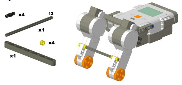
Slide the 12 stud axle through the mounting beams of the motor and secure it in place with  $\frac{1}{2}$  bushings. Use the friction pins to attach the 13 hole beam across the tops of the motors.
