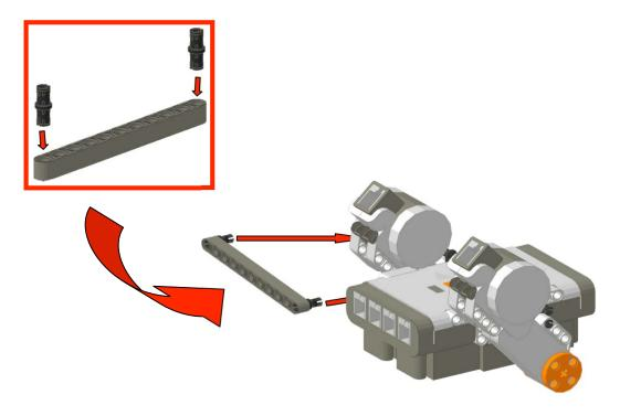
Take an 11-holed rounded beam and attach two short black connector pegs to the outside holes as seen in the red square. Connect the pegs to the back of each motor (as identified by the red dots) to further support the motors to the NXT. Your NXT should look like the below picture before moving on to the next step.
