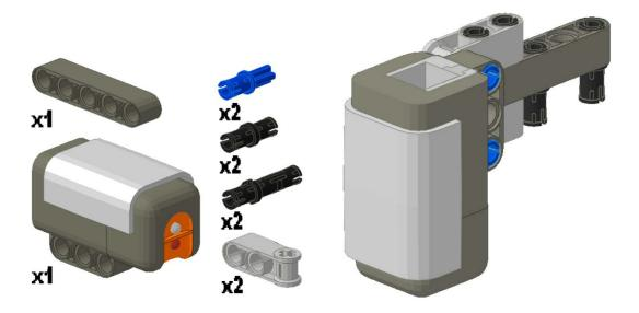
Insert a black connector peg into the 1st and 3rd holes of the 5-hole beam and an extended black connector peg into the 4th and 5th holes. Attach an axle joiner to the extended black connector pegs. Insert a friction axle into each hole of the axle joiners and attach the light sensor to the friction axles. Attach the light sensor to the car from Step #5. The 5-hole beam should connect to the top of the L-beam on the front wheel assembly.
