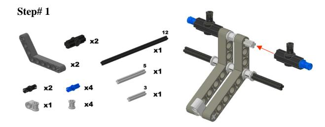
Attach to the side of each angle connector an axle pin. To the top of each, connect a pin. Thread a medium axle between the angle connector placing 2 bent beams and a bushinging in between. At the bend of the beams, thread a long axle with bushingings inside and outside of the beams. At the end of the beams, thread a small axle with a perpendicular axle joiner.
