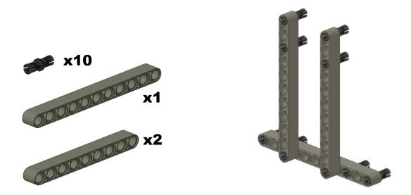
Separately build a motor support using beams and pegs.
