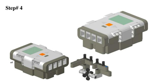
Attach the parts from Step# 3 to the NXT at the protruding connector pegs.
