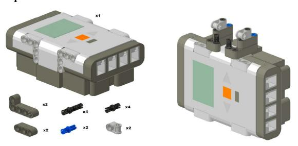
Build the NXT assembly. Attach a series of beams and pegs that will allow you to attach the top portion of the merry-go-round.
