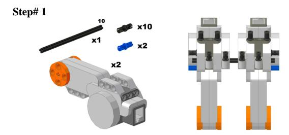
Attach 4 pins to the back of 2 motors. Also attach a pin and an axle pin to the side of each motor. Take 4 pins and attach each to a perpendicular axle joiner. Thread an axle through each motor lining up the 4 perpendicular axle joiners.
