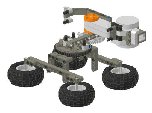
Attach the base motor assembly to the base. Remove the 40-tooth gear and thread the axle through the 4 pin connector.
