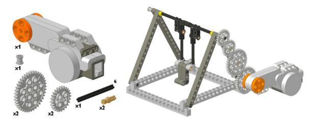
Place 1 of the 24-tooth gears on the exposed 10-stud axle at the top of the assembly. Connect the other 24-tooth gear using the axle pin to the  $4^{th}$  hole from the top of the beam. Connect one of the 40-tooth gears to the  $8^{th}$  hole from the bottom of the beam. Connect the other 40-tooth gear to the  $2^{nd}$  hole from the bottom of the beam using the 6-stud axle to the motor. Secure the motor in place with a bushing.
