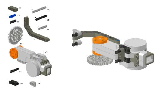
Build the base motor assembly. Attach to the motor a series of beams and pegs. Also thread an axle through the motor and attach a 40-tooth gear.
