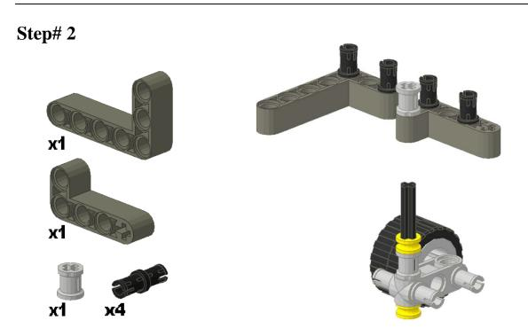
Take a small L-beam and attach 2 black friction pins to the 2nd hole and the 2nd hole from the top. Attach that to the parts from Step# 1 with a bushing. Take an L-beam and attach 2 black friction pins to the 2nd and 3rd holes.
