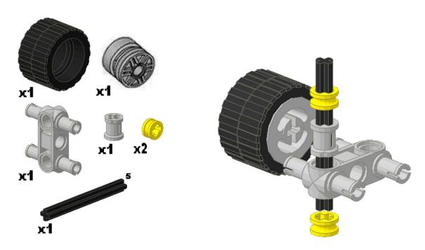
Take a 5 stud beam and slide on a half bushings, a 4-connector peg, a bushing and another half bushing. Attach the wheel to the 4-conector peg.
