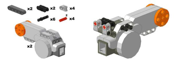
Connect 2 gray axle joiners to the black axle joiner using two 2 stud axles. Connect the 5 hole beam to the gray axle joiners using a long friction pin. Then connect the beam to the motor using 2 more long friction pins. Repeat this process for the 2nd motor.
