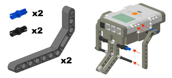
Secure the assembly by attaching a bent beam to each side of the NXT threading the long axle and the axle pin to the bent beam.
