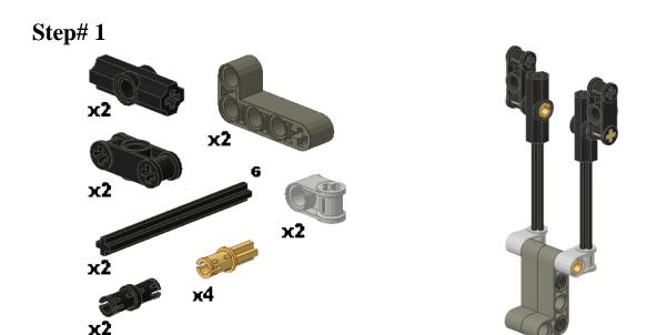
Connect the 2 lift arms using 2 axle pins. Place an axle pin with friction into the top holes of the lift arms. Connect these pins to the gray axle joiners. Insert a 6 stud axle into each axle joiner. Place a gray connector on each axle. Connect the black axle joiners using the 2 stud axles.
