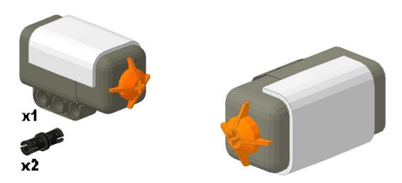
Attach the two black connector pegs to the first and third holes of the touch sensor. Attach the touch sensor assembly to the car from Step #5. The sensor should attach to the top of the L-beam on the front wheel assembly.
