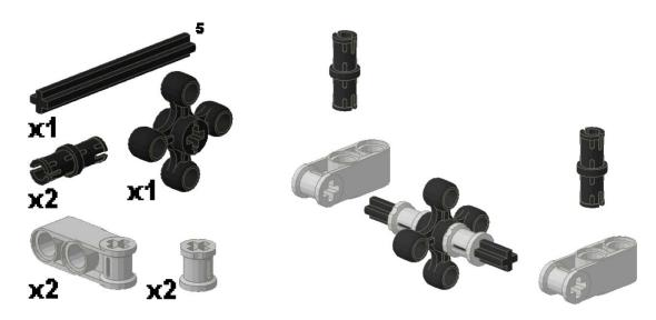
Slide a 5 stud axle through the skid. Side on 2 half bushings to keep the skid centered followed by 2 axle joiners on each end. Place a friction pin into the middle hole of the axle joiners.
