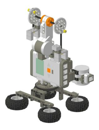
Attach the 2 horses to the 12-axle of the top motor assembly. Wire the motors to the NXT outputs and your merry-go-round is complete.
