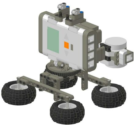
Attach the NXT assembly to the base and base motor. The NXT should attach in 3 places on the base and 4 places on the motor.
