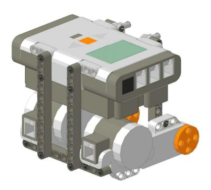
Attach the part from Step #1 to the part from Step #2 so that the beams from the first step connect to the back of the motors.
