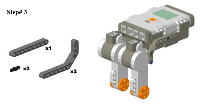
Attach 2 pins to the side of the NXT. Secure Step #2 by attaching a bent beam on both sides of the NXT and a straight beam on top of each motor.
