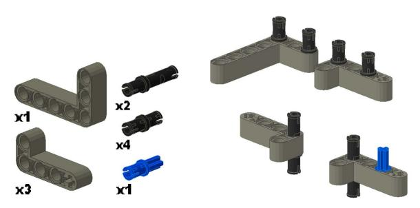
Take 2 small L-beams and place an extended black friction pin through the 2nd hole. On one of these small L-beams place a blue axle pin in the 2nd hole from the top. Take another small L-beam and insert 2 black friction pins in the 2nd hole and the 2nd hole from the top. Take an L-beam and insert 2 black friction pins into the 1st and 3rd holes.
