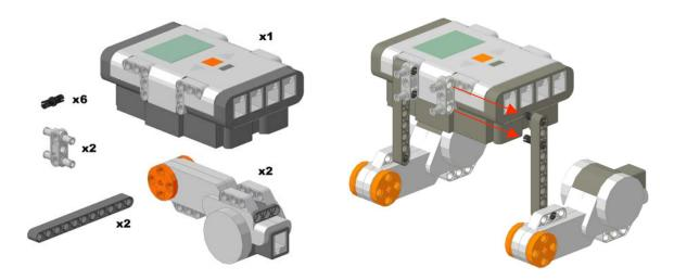
Attach 2 motors to the NXT using beams and various pegs.
