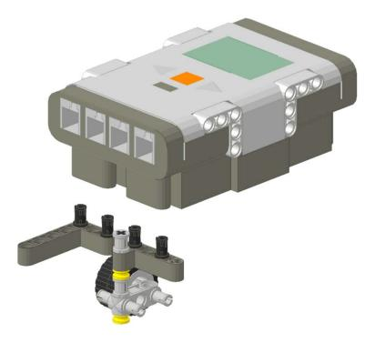
Attach the parts from Step# 2 to the NXT at the protruding connector pegs.
