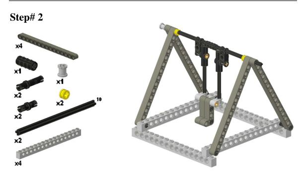
Slide the 10 stud axles through the gray axle joiners from the previous step, and connect them using the axle connector. Create the base by connecting the beams to the 1st and 15th hole of the studded beams using a pin and a long pin. Reinforce the base by connecting 2 more studded beams to the bottom of the frame. Slide the 10 stud axles through the ends of the beams and secure in place with one bushing and two ½ bushings.
