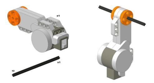
Assemble the top motor assembly. Thread a 12-axle through the motor.
