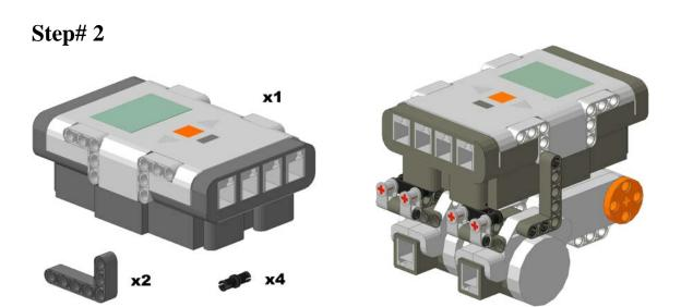
Attach each motor assembly to the bottom of the NXT by the black axle joiner, using a friction pin. Then secure each motor using the bent beam.
