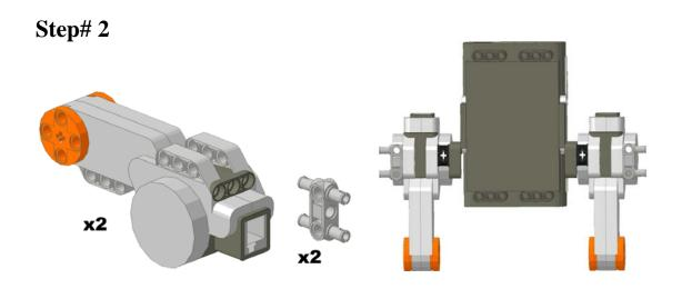
Fasten the motors to the double pin connectors on the bent beams. Then fit a 4 pin connector into the outside mounting beam on the NXT.
