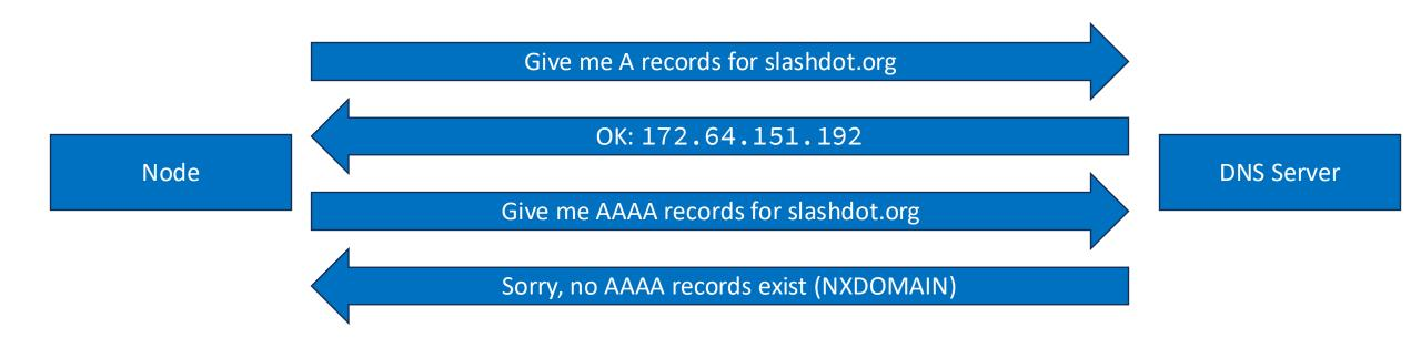
Node only receives IPv4 addresses, so communicates over IPv4
