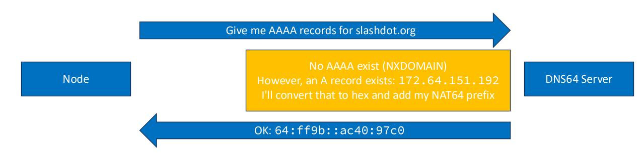
Node receives IPv6 answer, proceeds normally. Packets are routed to NAT64 PLAT which handles translation to IPv4 for delivery.
